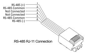
Illustration 2: Modbus™™ Cable Wiring
