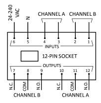
\* On 1-wire seal-fail circuits attach Pin 4 to COMMON GROUND point with PUMP SAFETY GROUND WIRE.
